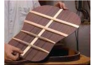
The bracing on the inside of the guitar's rosewood back provides structural support to compensate for the channel cut for the marquetry inlay and for the curve of the guitar's back surface.
