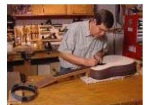
Lynn Dudenbostel measures and marks the precise placement of the fingerboard on the neck of the guitar.
