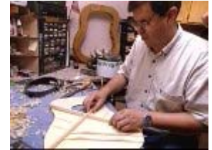
Lynn Dudenbostel places the bracing and tone bars on underside of the guitar top. Luthiers refer to this critical step in the guitar-making process as "giving voice" to the guitar.
